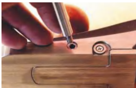
▲ The fence bars screw in securely to tapped holes in the body
